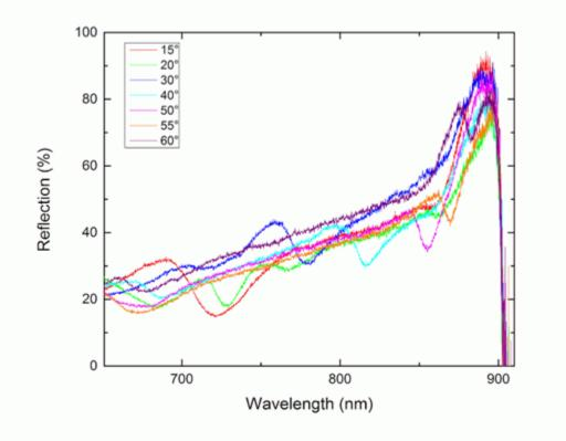
2. We etch the sample photonic crystal sensor to characterize that the best performance wavelength is surely at 845nm. The sensor is good enough for our usage for detection.
